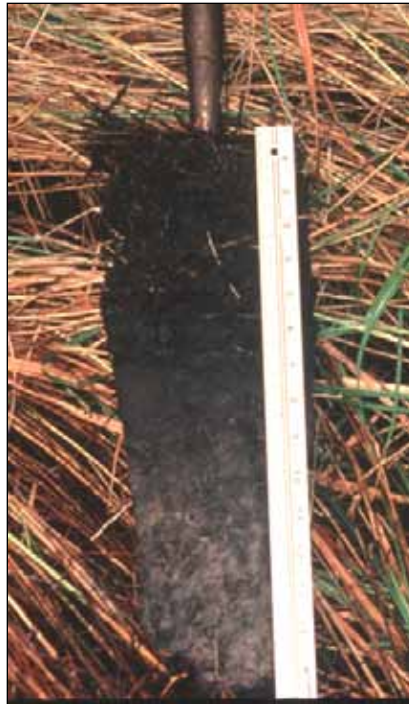
Figure 14. The mucky modified sandy layer is approximately 3 in. (7.5 cm) thick. Scale in inches on the right side of ruler.
